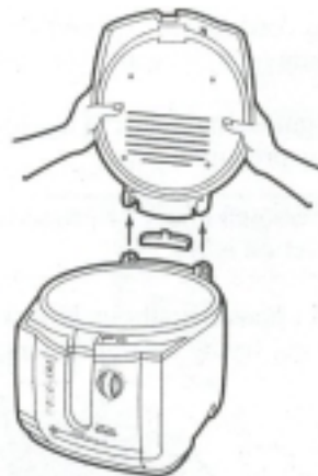
Diagram 5 Open cover 90°, lift to remove Lift condensation cup to remove
