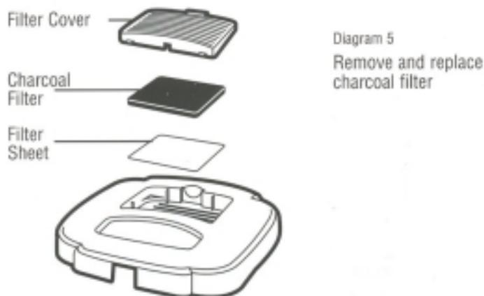
To replace charcoal filter, push in release clip on filter cover. Lift charcoal filter out and discard. Wipe recess area clean with a damp soapy cloth, wipe clean and dry. Wash filter cover in hot soapy water, rinse and dry. Place new charcoal filter into recess with thin filter sheet down first. Replace filter cover and close to lock in place. See Diagram 5.
